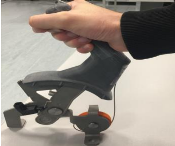
Figure 2. Prototype of the designed hand brake with additive manufacturing
