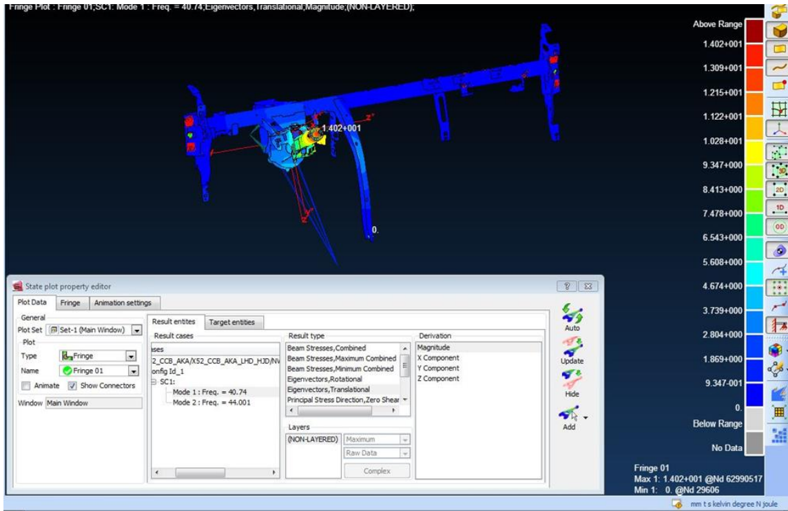
Figure 4. NVH HJD Type Steering Analysis, 1st and 2nd Natural Frequency Values
